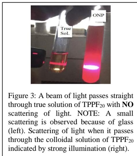
Figure 3: A beam of light passes straight through true solution of TPPF<sub>20</sub> with **NO** scattering of light. NOTE: A small scattering is observed because of glass (left). Scattering of light when it passes through the colloidal solution of TPPF<sub>20</sub> indicated by strong illumination (right).
