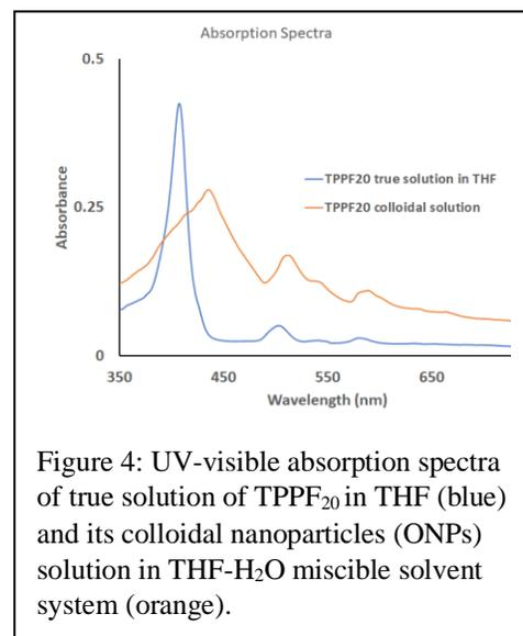
Figure 4: UV-visible absorption spectra of true solution of TPPF<sub>20</sub> in THF (blue) and its colloidal nanoparticles (ONPs) solution in THF-H<sub>2</sub>O miscible solvent system (orange).
